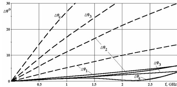
Figure 3. Measured phase characteristics of attenuator as function of frequency
