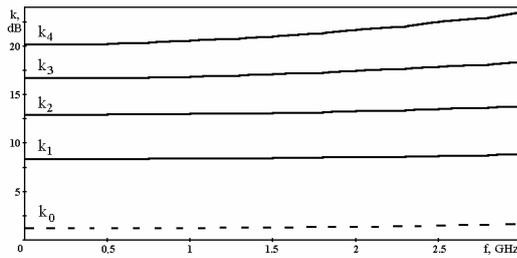
Figure 2. Measured attenuation characteristics as function of frequency
