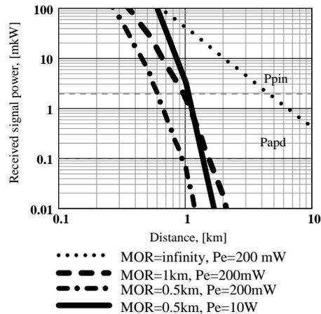
Fig. 1. Received signal power at receiver lens of the operation distance depending of fog density at: output power 200 mW, transmit beam divergence 10 mrad, receiver lens diameter 100 mm, sensitivity 2 mW
