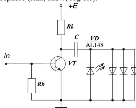
Fig.2. The last cascade of the high power transmitter
